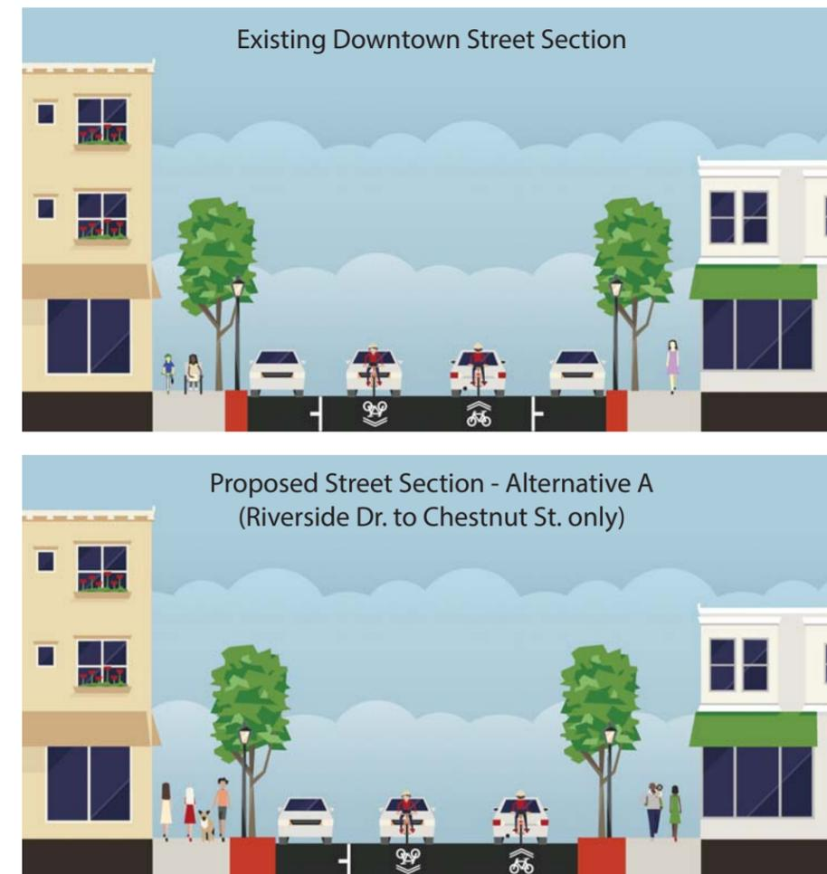
Figure 6: Existing vs. Proposed Street Sections
