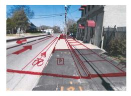
Figure 9: Sketch of proposed sidewalk improvements on the east side of Spring Street north of Riddle St. By reclaiming the paved ROW on the building side of the concrete gutter we can reintroduce parallel parking in this segment.
